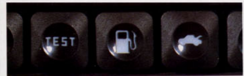
Service test control switch (by pushing switch, all warning lights light up. Should one of the warning lights not light, relevant bulb or electric circuit is faulty). Fuel tank flap opening power switch Trunk release power switch
